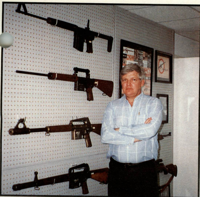
Reed Knight poses in front of the four evolutionary prototype models of the AR-10. From top No. 1 in caliber .30-06 with BAR magazine and Johnson rear sight; No. 2 in caliber 7.62/.308 with telescopic sight; No. 3, the "AR-10A" and No. 4 the definitive American AR-10. History really does repeat itself! Reed's pose in the photo is the same pose made by Gene Stoner himself for Guns Magazine back in 1957.
