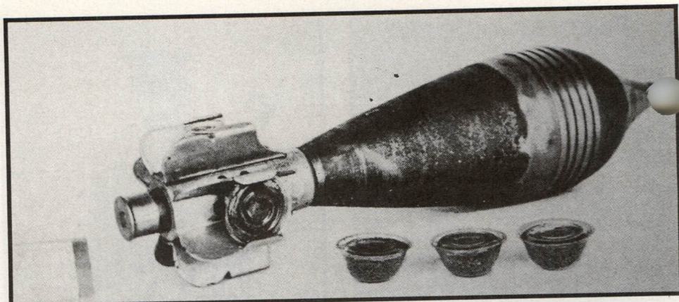
Prototype ammunition for Model 1927. Note "zone charges," used for setting pattern dispersion.
