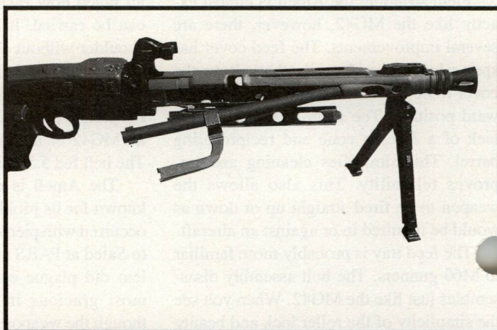
Barrel removes from right side.
